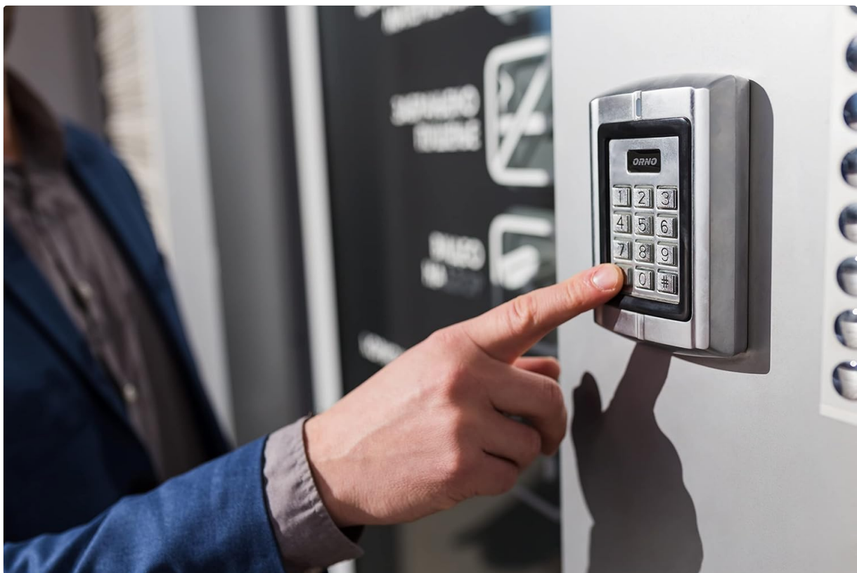
Figure 4.1: A user interacting with the illuminated keypad of the Orno ZS-802 to enter an access code.
