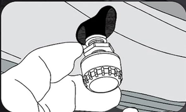
3. Tighten the nut to hold on sensor with anticlockwise.
