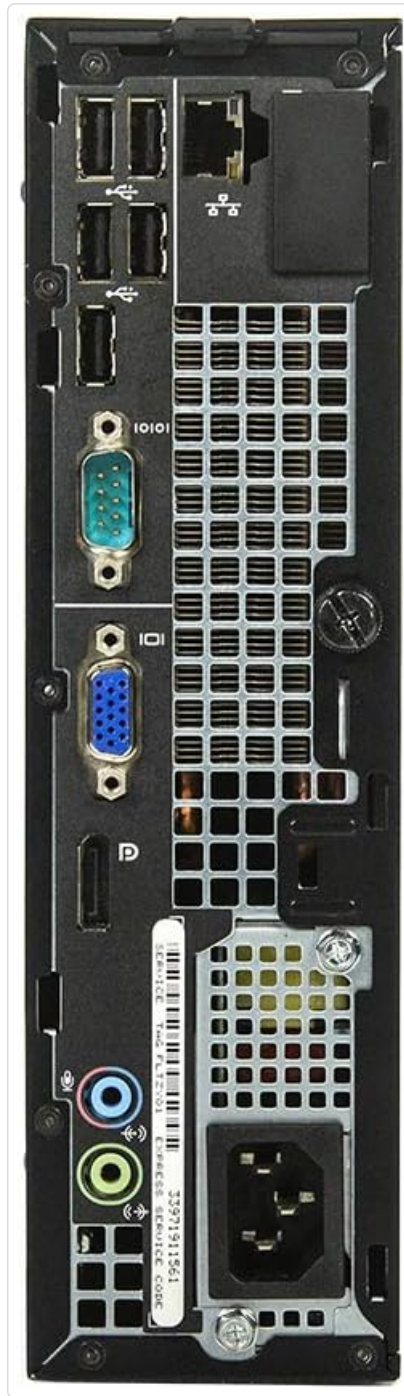
Image: Rear view of the Dell Optiplex 780 USFF desktop PC, highlighting the available ports.
