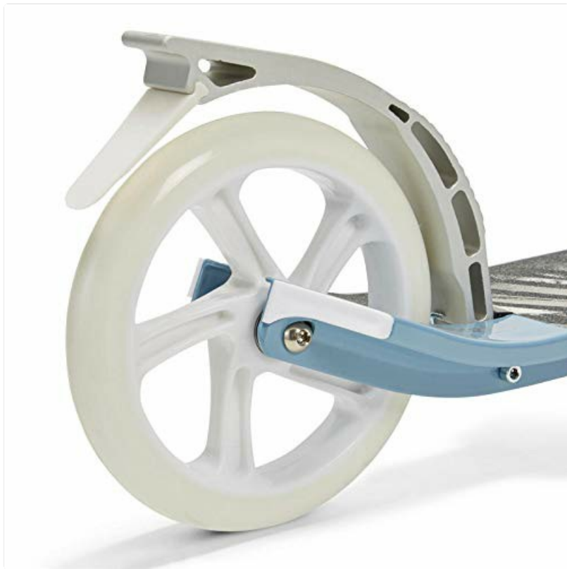
Figure 5: Detail of the rear wheel and fender brake.
