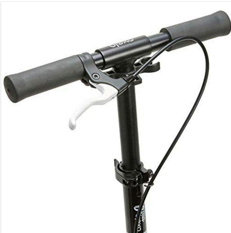
Figure 2: Detail of the adjustable handlebar and ergonomic grip with the brake lever.
