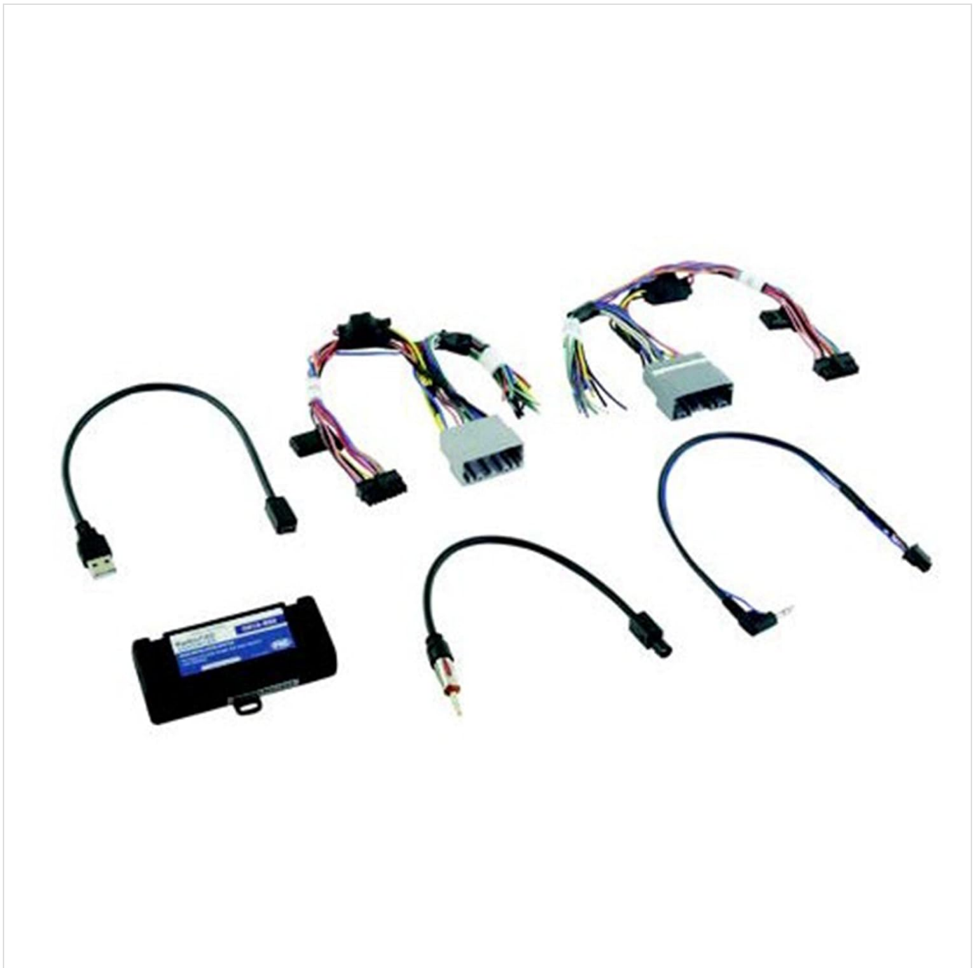
Figure 3.1: Contents of the PAC CH1A-RSX package. This image displays the central PAC interface module, two distinct multi-pin wiring harnesses for vehicle integration, a USB cable for potential firmware updates or configuration, and two additional smaller adapter cables, likely for specific audio or data connections.
