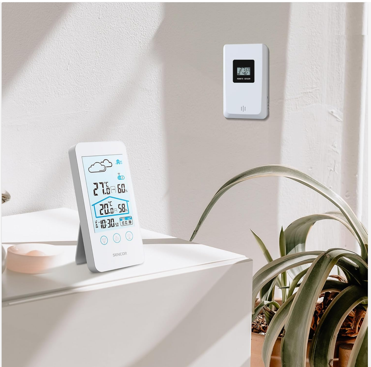
Figure 5.2: The main unit can be placed on a flat surface, while the sensor is mounted on a wall or suitable outdoor location.
