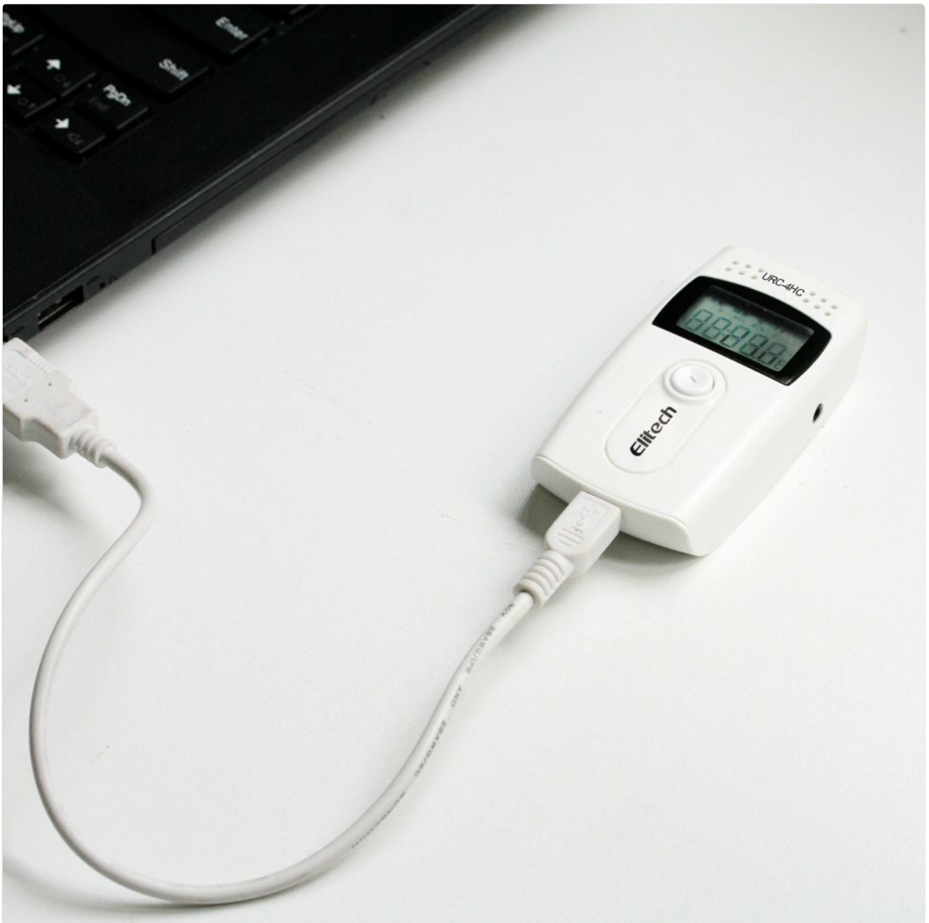
Image 4: The Elitech RC-4HC data logger connected to a computer via USB and also showing the external temperature sensor connected.
