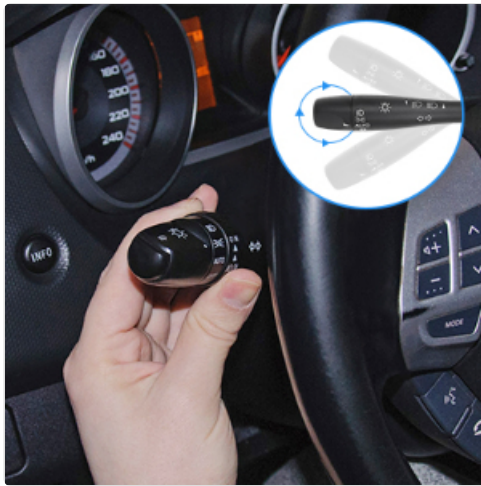
Image: A hand demonstrating the operation of the turn signal switch lever.
