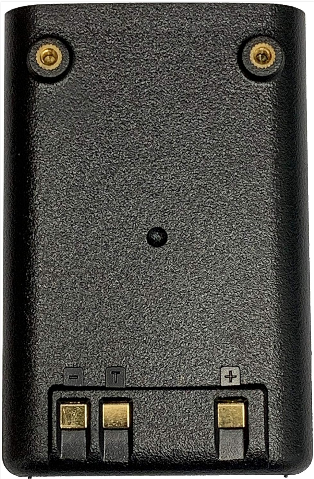
Figure 3.2: Rear view of the ALINCO EBP-87 Li-ion Battery Pack. This side shows the three main connection terminals: negative (-), temperature (T), and positive (+). These terminals facilitate charging and power delivery to the compatible radio device. Two screw holes are visible at the top for secure attachment to the radio.
