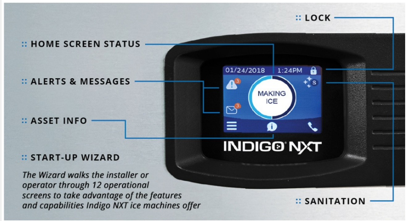
Figure 5: Indigo NXT display with labeled functions including Lock, Home Screen Status, Alerts & Messages, Asset Info, Start-Up Wizard, and Sanitation.
