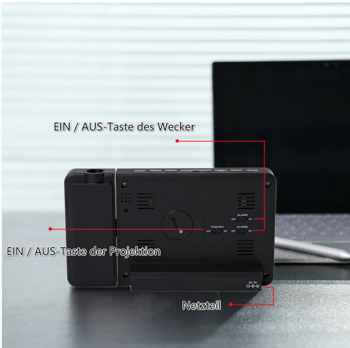
Image: Rear view of the main unit, highlighting the power input and various control switches.
