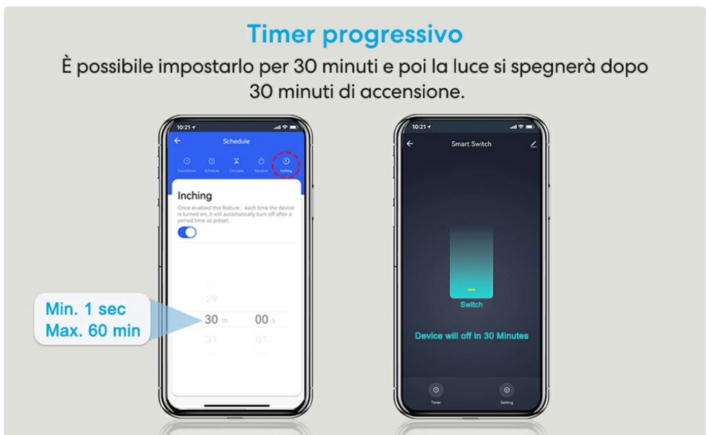
Image: Screenshot of the Smart Life app showing the 'Inching' timer setting, allowing users to set a duration for automatic turn-off.
