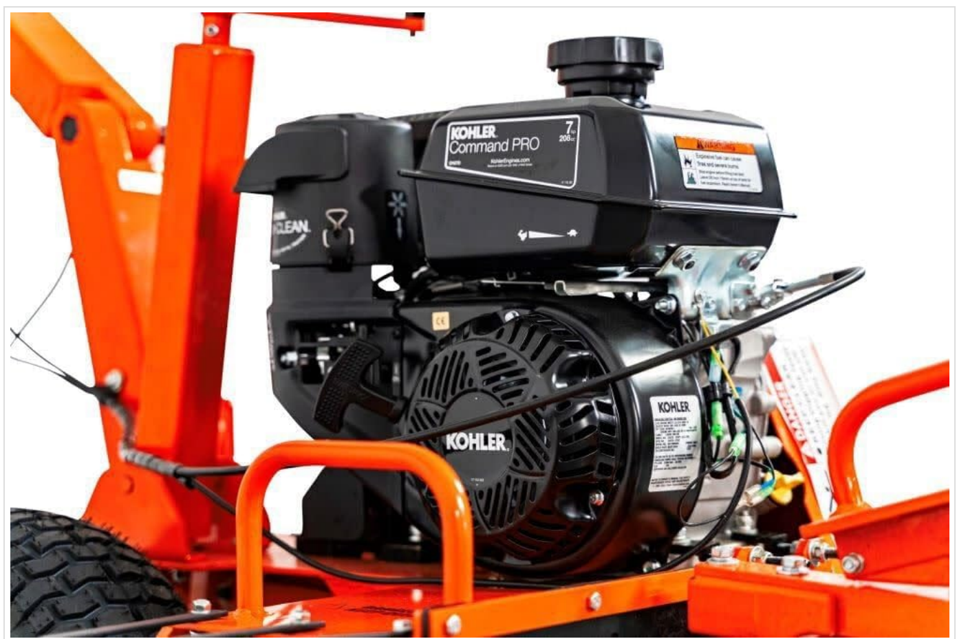
Figure 5: Detailed view of the Kohler 7HP engine, showing key components for maintenance access.
