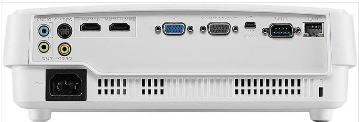
Image 2.2: Rear panel of the BenQ MX707 DLP Projector, displaying connectivity ports.
