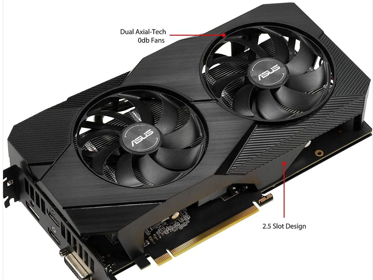
Figure 4.3: Top view illustrating the dual axial-tech fans and the 2.5 slot design for enhanced cooling and compatibility.
