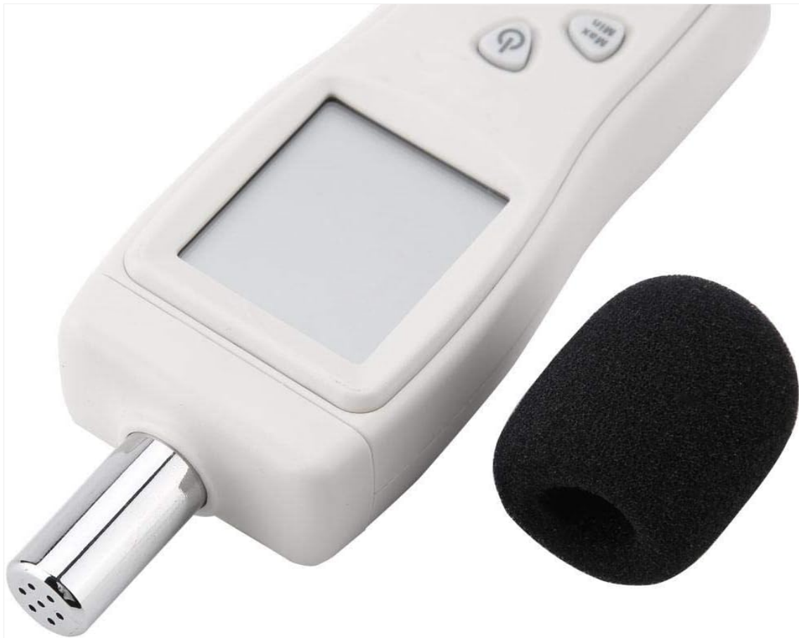
Figure 3.2: Close-up view of the microphone with the windproof ball removed.
