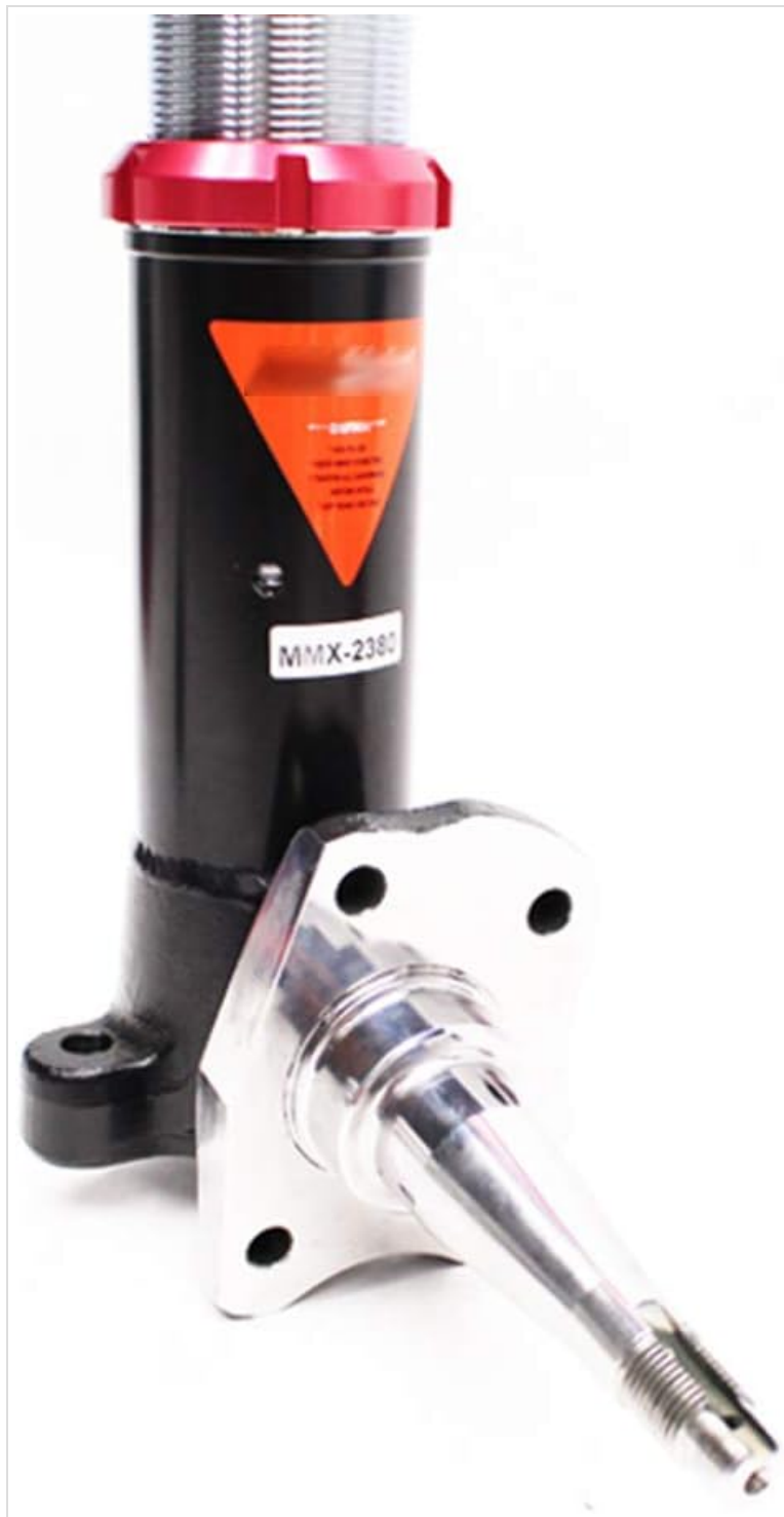
Figure 3.7: The front coilover's lower mount integrated with the spindle, demonstrating the direct fitment design.
