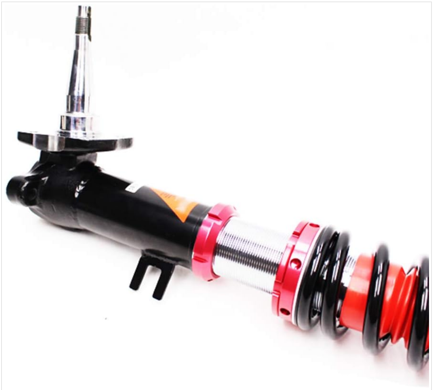
Figure 3.8: Another perspective of the front coilover, highlighting the spindle and lower mounting points for secure installation.
