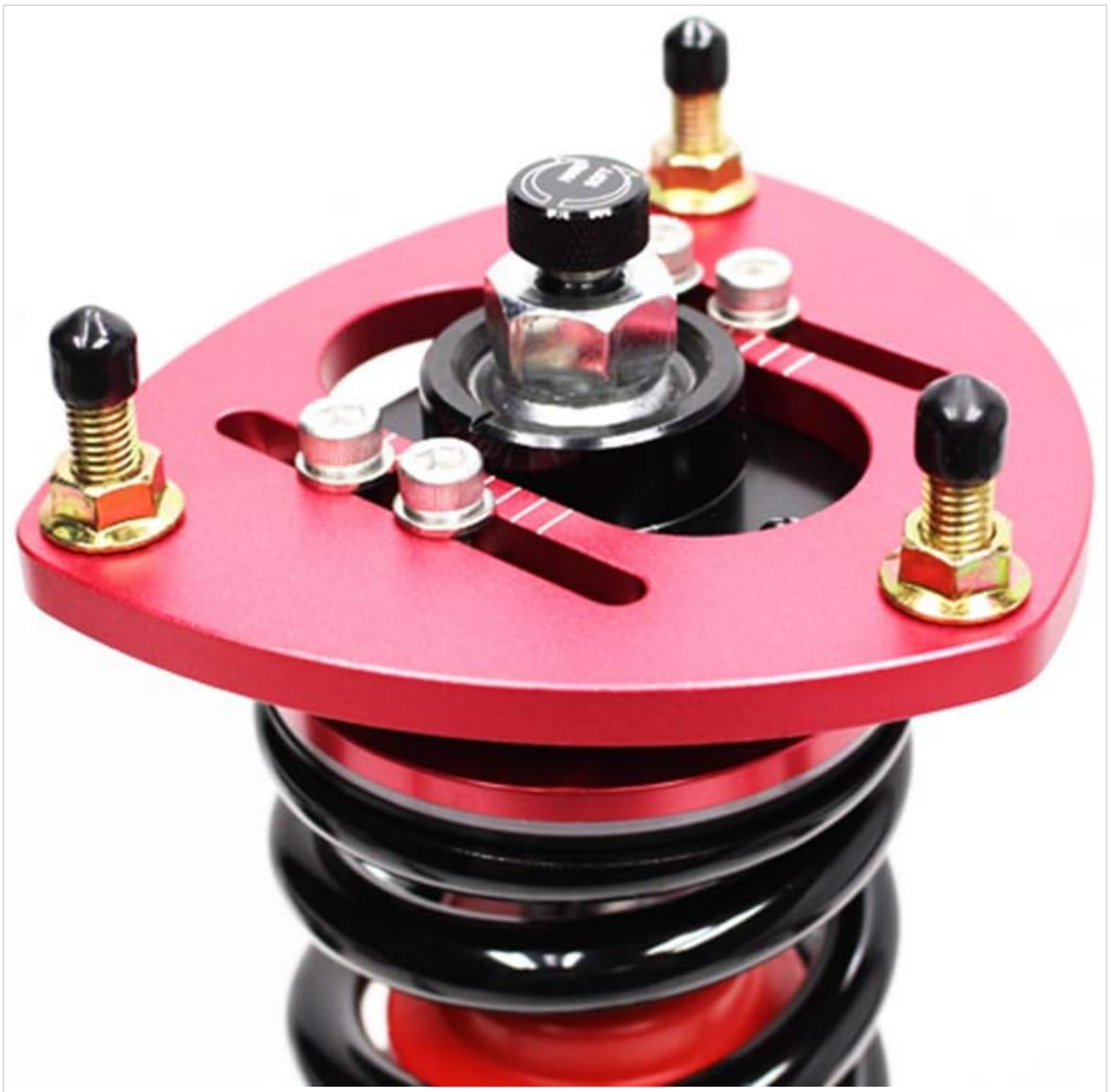
Figure 3.3: Detailed view of the rear coilover's standard top mount and damping adjustment knob.
