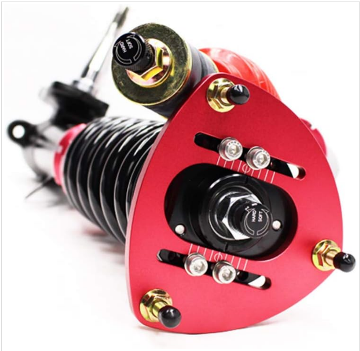
Figure 3.2: Detailed view of the front coilover's adjustable camber plate and damping adjustment knob, allowing for precise suspension tuning.
