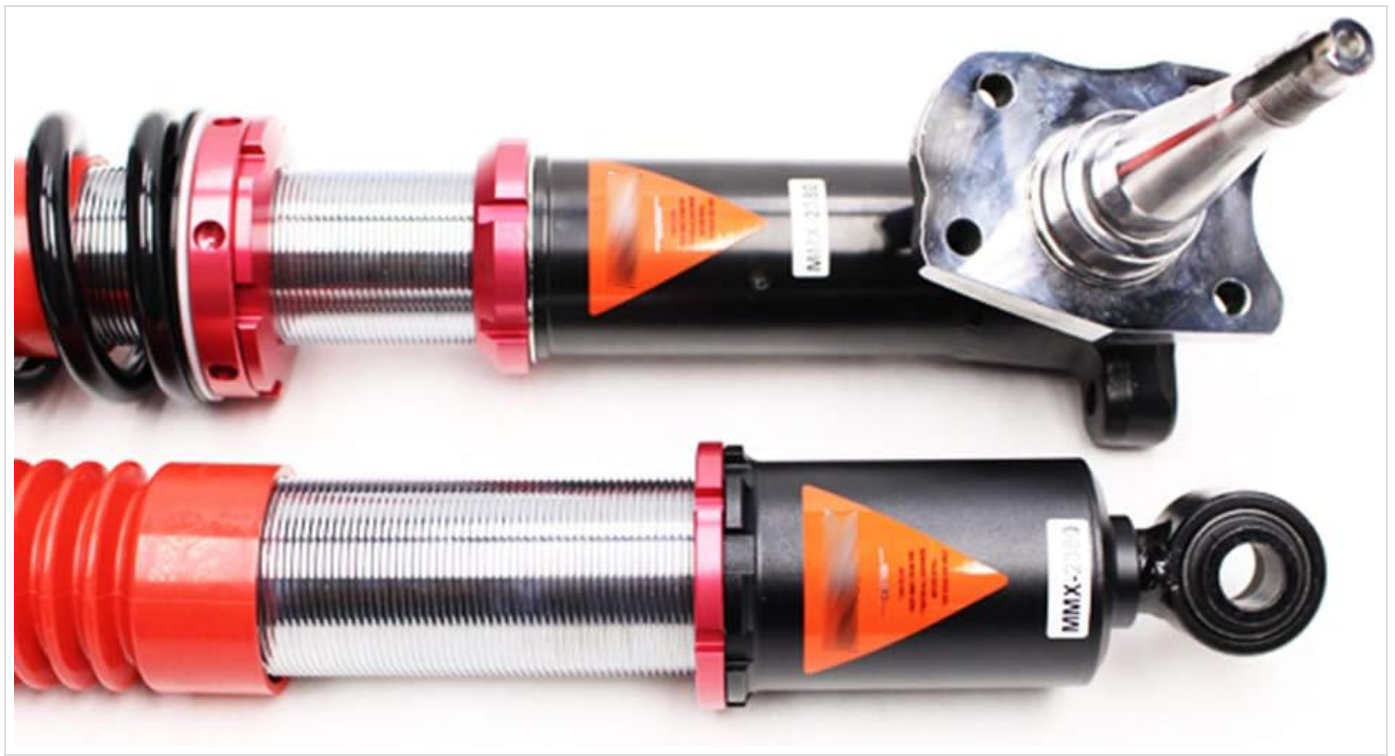
Figure 3.6: Close-up of the front coilover's main body and the robust lower mounting bracket.
