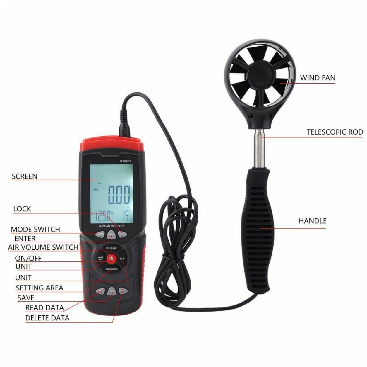
Figure 3: Detailed diagram of the GT8907 anemometer, highlighting the main unit's screen and buttons, and the wind fan probe with its telescopic rod and handle.
