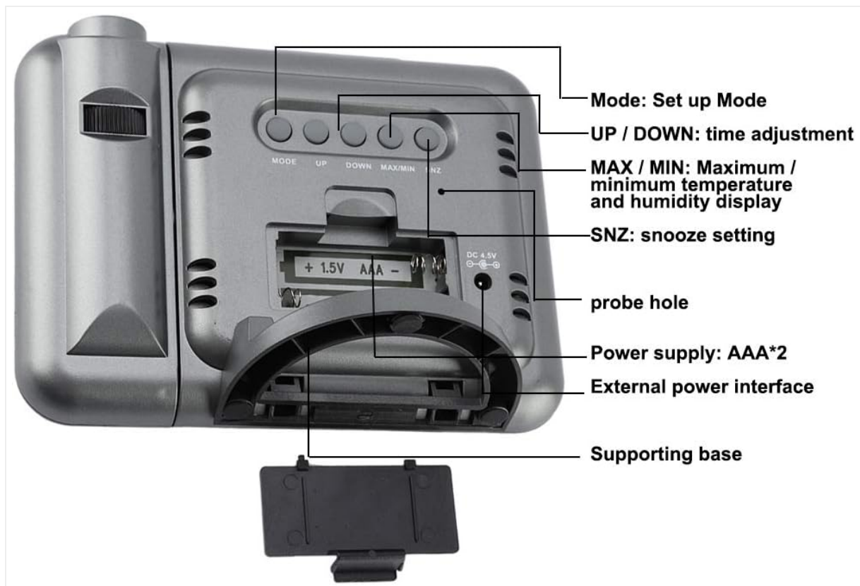
Figure 2: Rear view of the alarm clock, showing control buttons, battery compartment, and power input.
