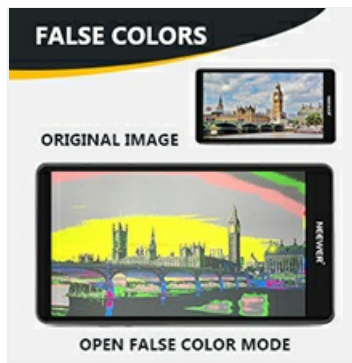
Figure 4.3: False Colors. This mode helps in evaluating exposure by representing different luminance values with distinct colors.
