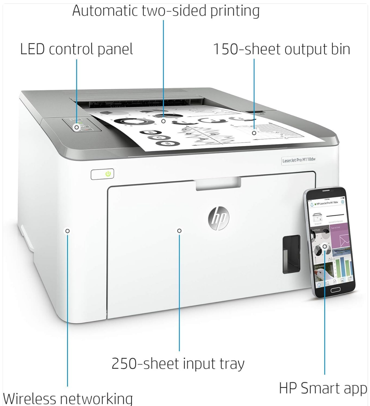
Figure 5: Key components of the HP LaserJet Pro M118dw printer.
