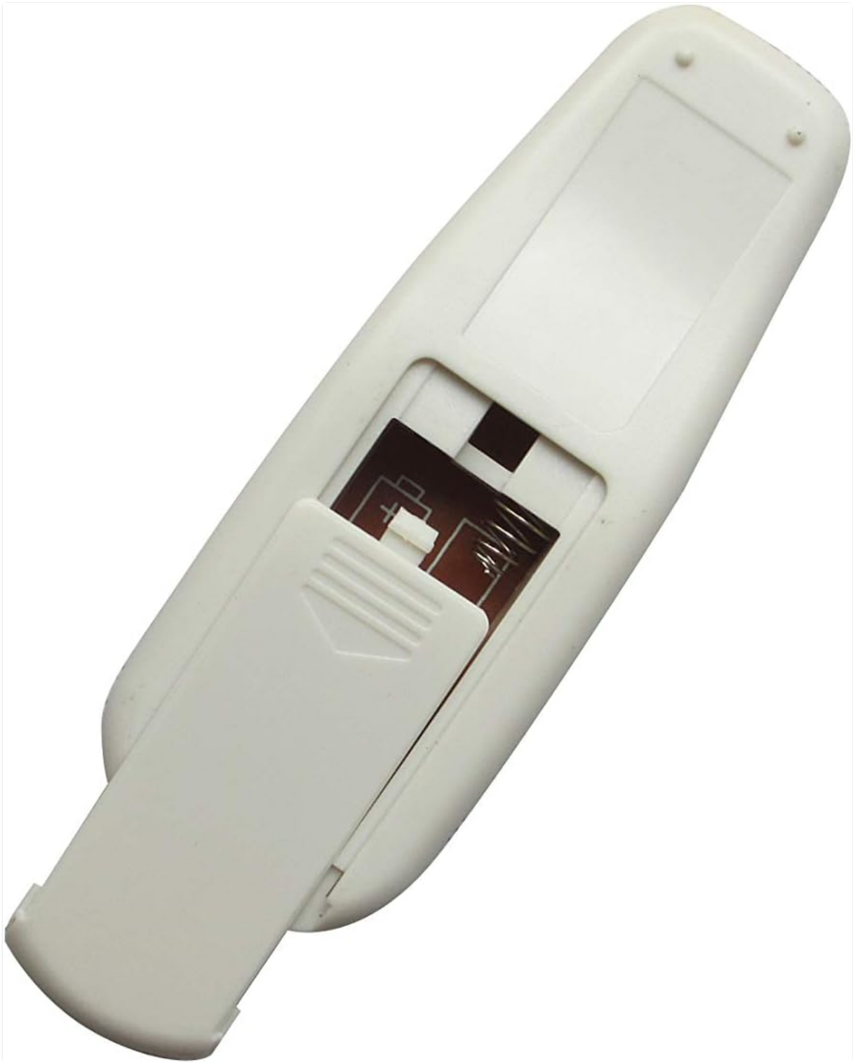
Figure 1: Battery compartment with cover removed, showing battery placement.
