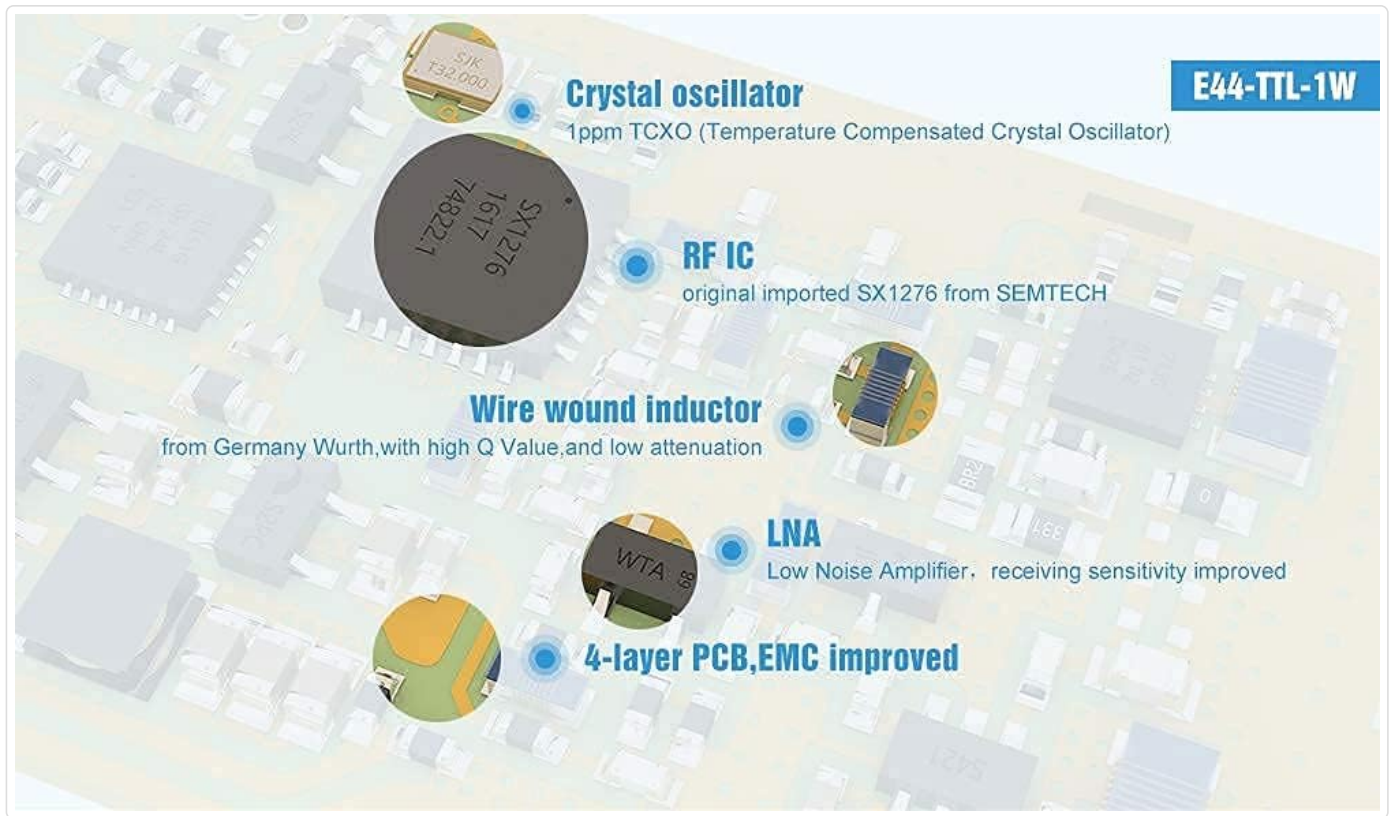
Figure 4: Key Internal Components. This image highlights the main components of the module, including the SX1276 RF IC, crystal oscillator, wire wound inductor, LNA, and the 4-layer PCB design.
