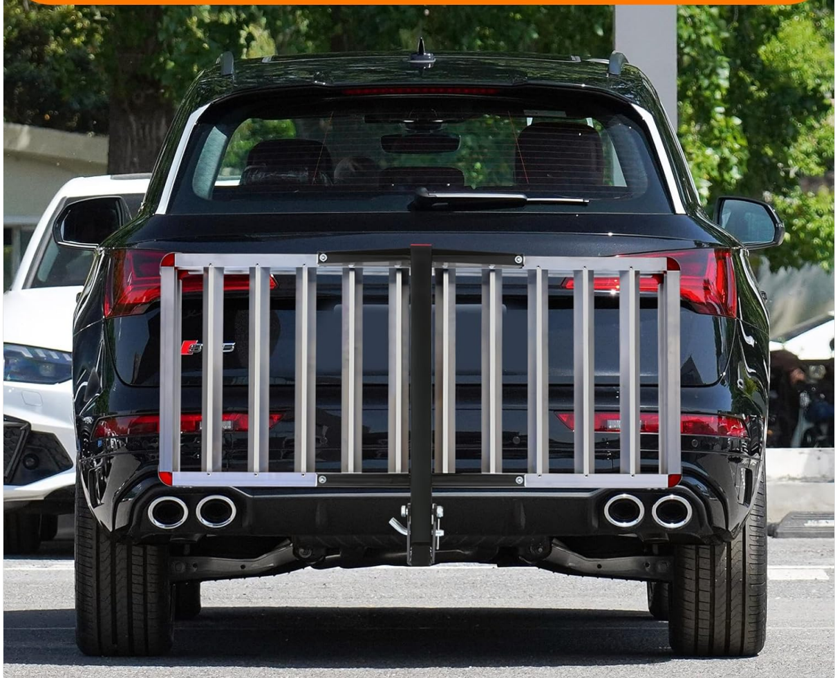
Figure 5.3: Carrier in Folded Position. This image demonstrates the carrier folded vertically against the vehicle for storage.
