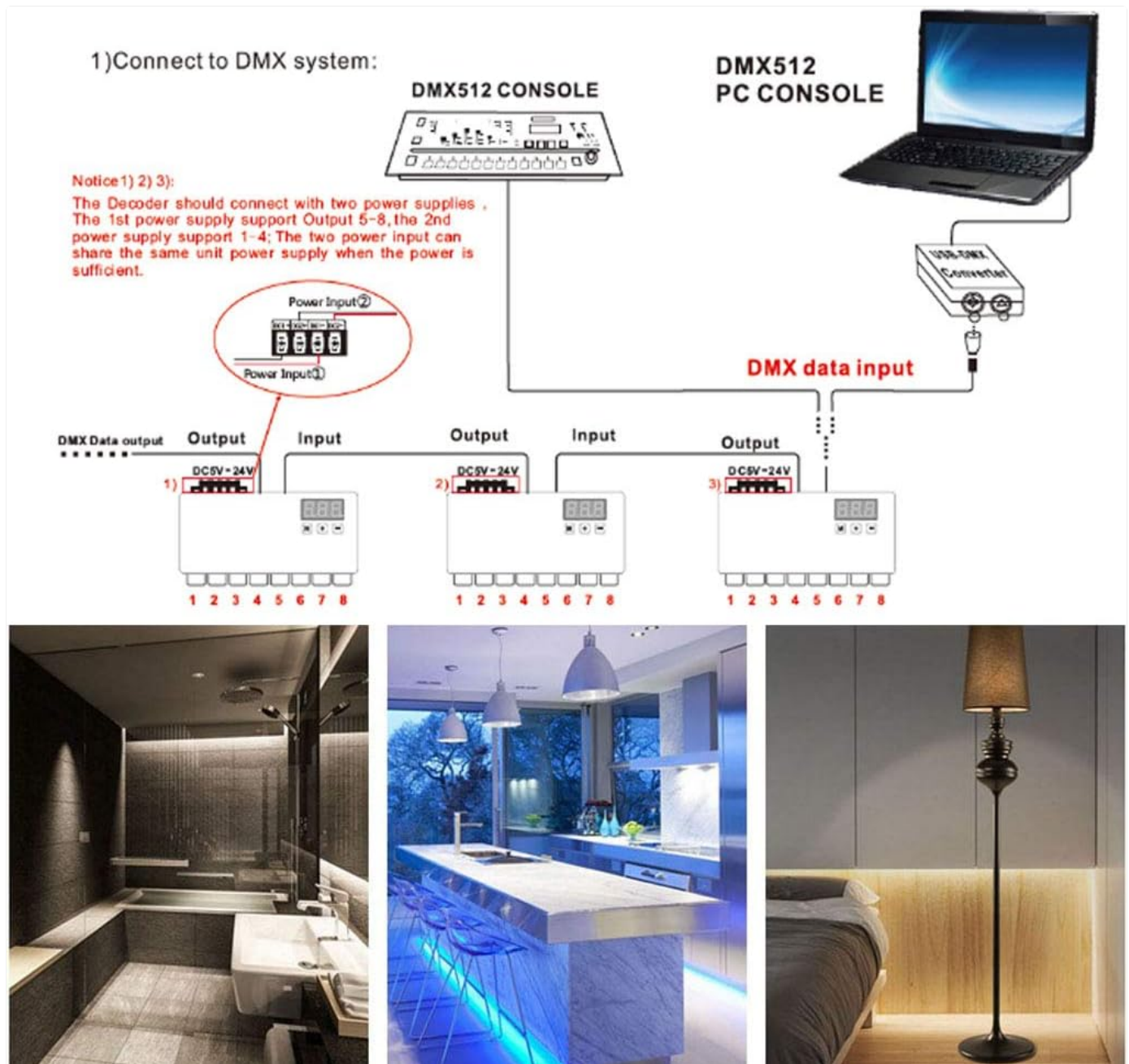
Figure 4.1: DMX512 system connection diagram. This diagram illustrates how to connect the DMX512 decoder to a DMX console or PC console, showing DMX data input, power input, and output connections to LED strips. It also highlights the use of two power supplies for different output groups.
