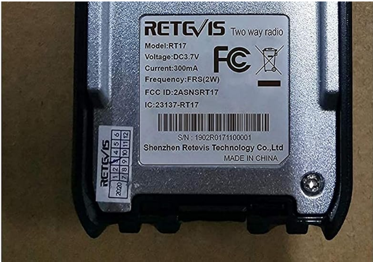
Image: The rear view of the Retevis RT17 radio, displaying its model information and FCC certification details.
