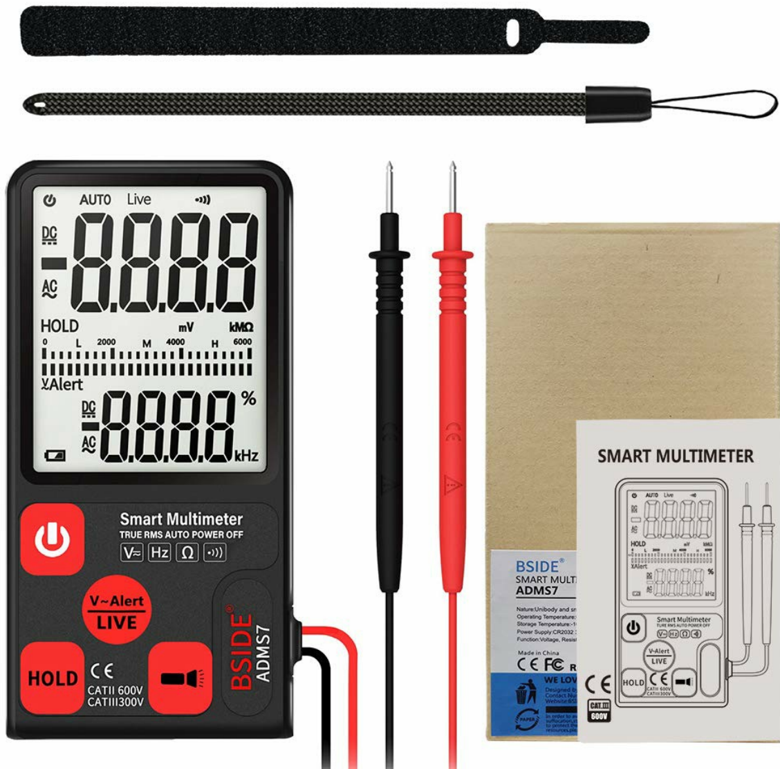
Figure 3.1: BSIDE ADMS7 Multimeter, including the main unit, red and black test leads, a wrist strap, and the product packaging.
