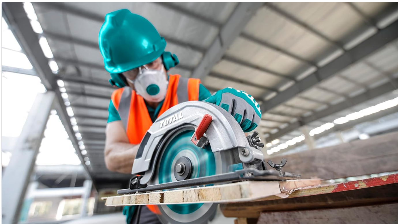
Figure 4: A user demonstrating safe operation of the circular saw, wearing appropriate personal protective equipment including a hard hat, safety glasses, and a dust mask.
