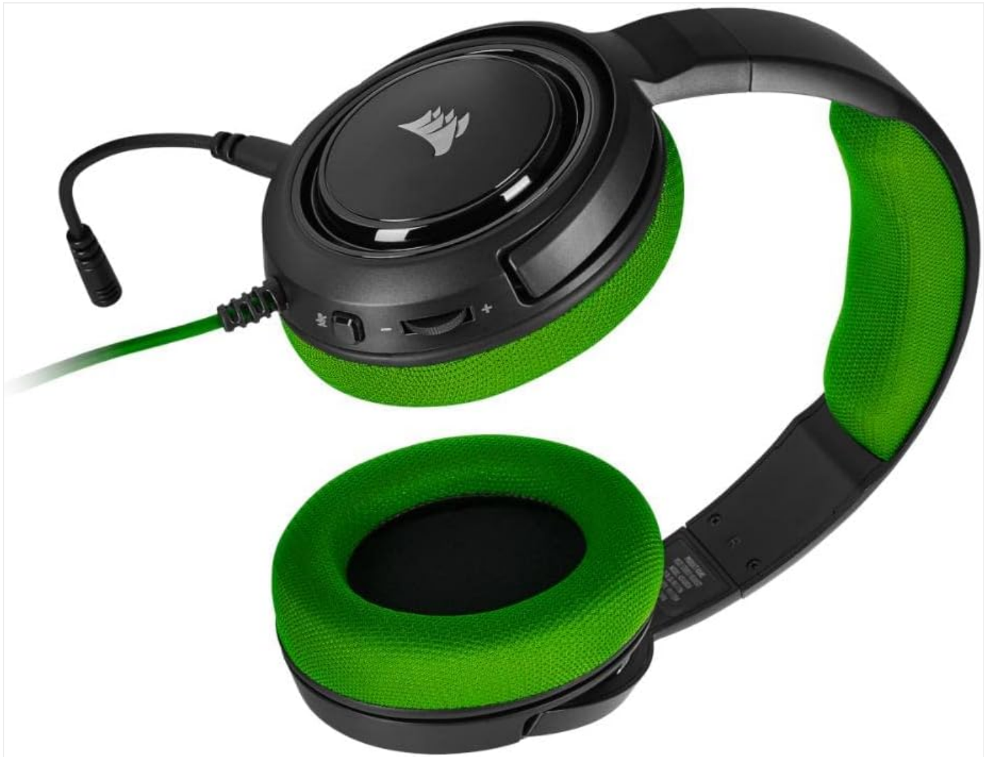
Image 3.2: View of the left earcup showing the 3.5mm audio cable and the microphone port.
