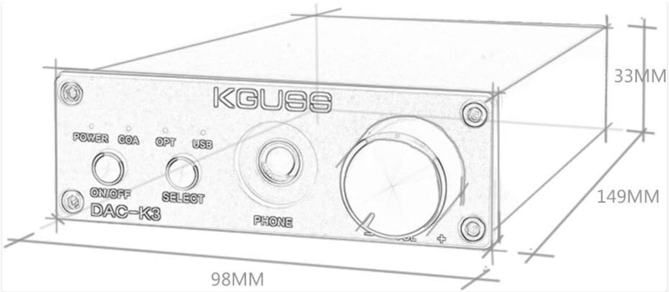
Image: Dimensional drawing of the KGUSS DAC-K3 unit.
