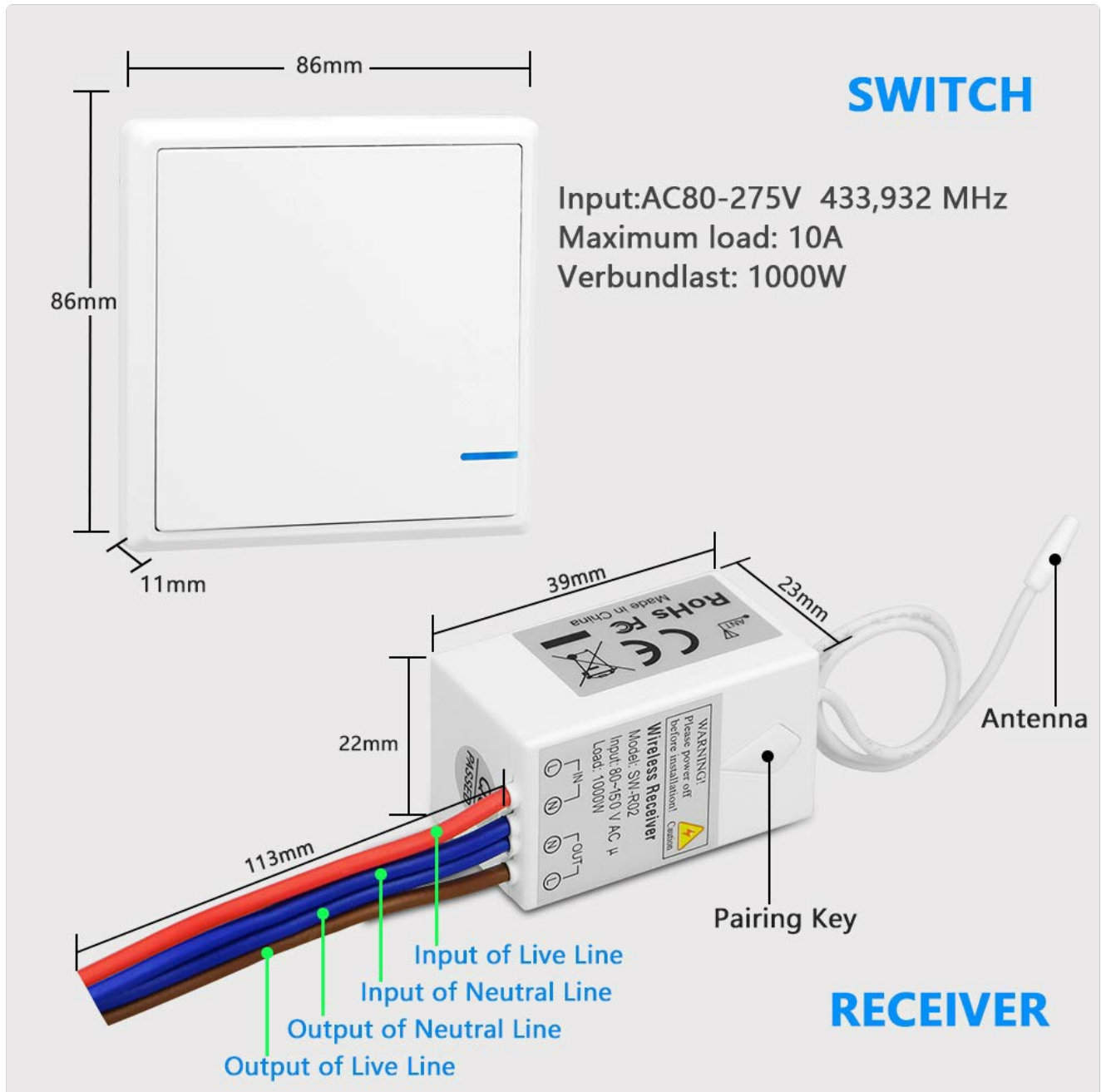
Image 3: Switch Dimensions and Receiver Wiring. This image displays the dimensions of the wireless switch panel (86mm x 86mm x 11mm) and the mini receiver (113mm x 39mm x 23mm). It also provides a clear wiring diagram for the receiver, showing connections for Input Live Line, Input Neutral Line, Output Neutral Line, and Output Live Line, along with the pairing key and antenna.
