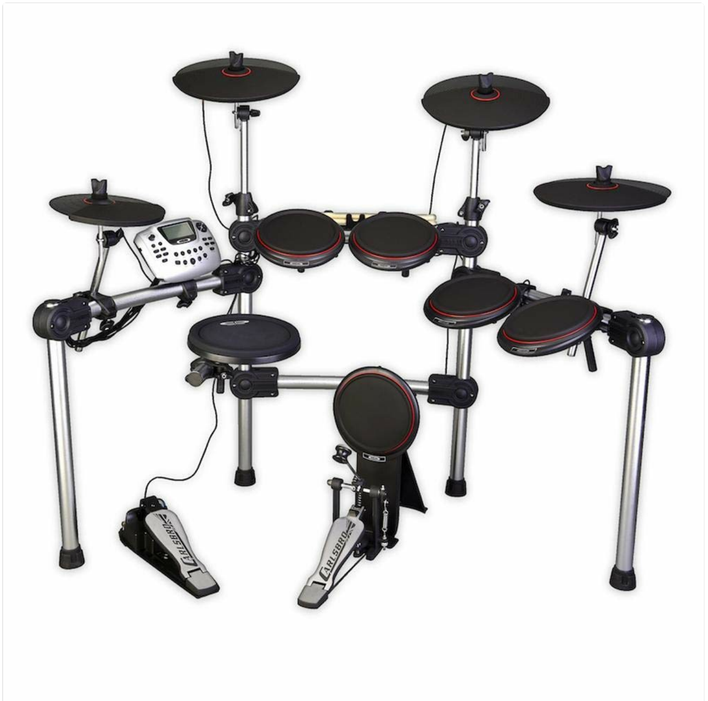
Figure 2.1: An overview of the Carlsbro CSD230 electronic drum kit, showing the drum pads, cymbals, sound module, and pedals mounted on its sturdy rack.
