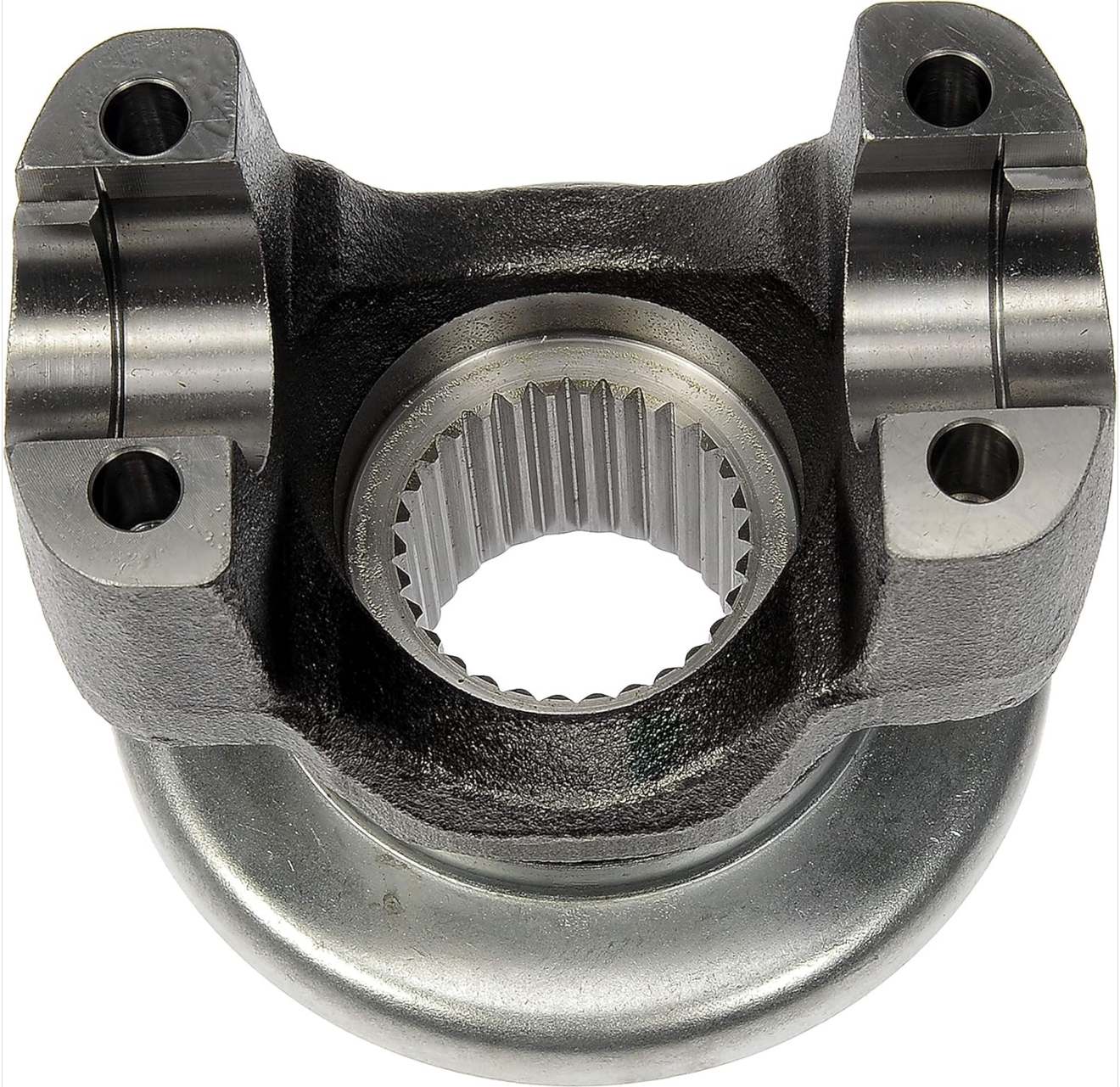
Image 2: Back view of the Dorman 697-551 Rear Differential End Yoke. This perspective highlights the splined bore where the yoke connects to the differential pinion shaft, and the U-joint strap bolt holes.
