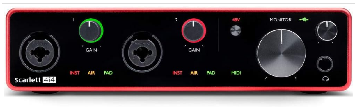
Figure 2: Front panel of the Scarlett 4i4 3rd Gen, highlighting input and control knobs.
