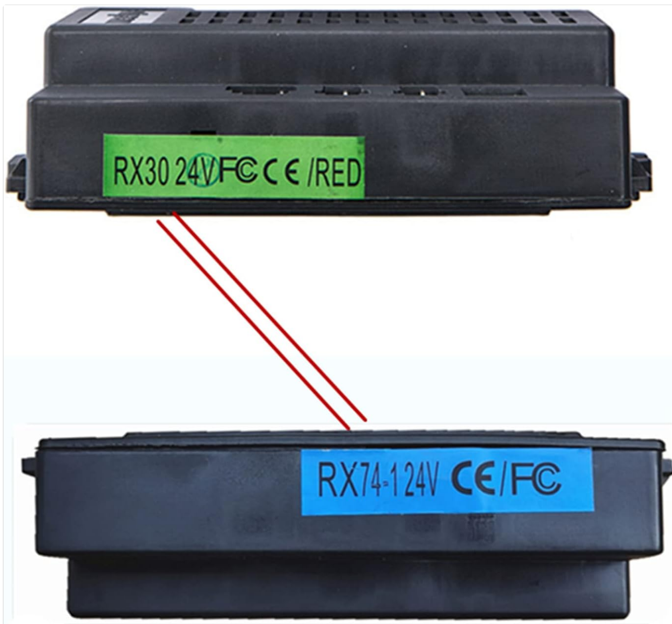
Image: Comparison of RX30 and RX74 control boxes, highlighting their interchangeability.
