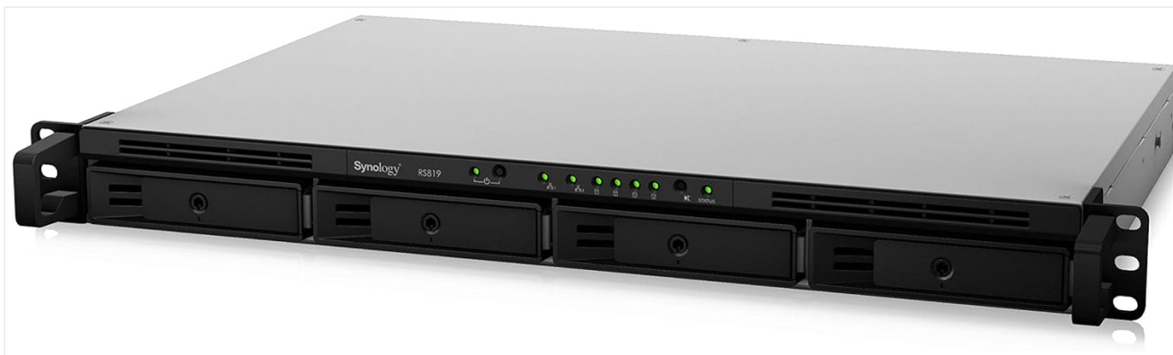
Figure 3: Angled view of the Synology RS819, illustrating the accessible drive bays for hard drive installation.
