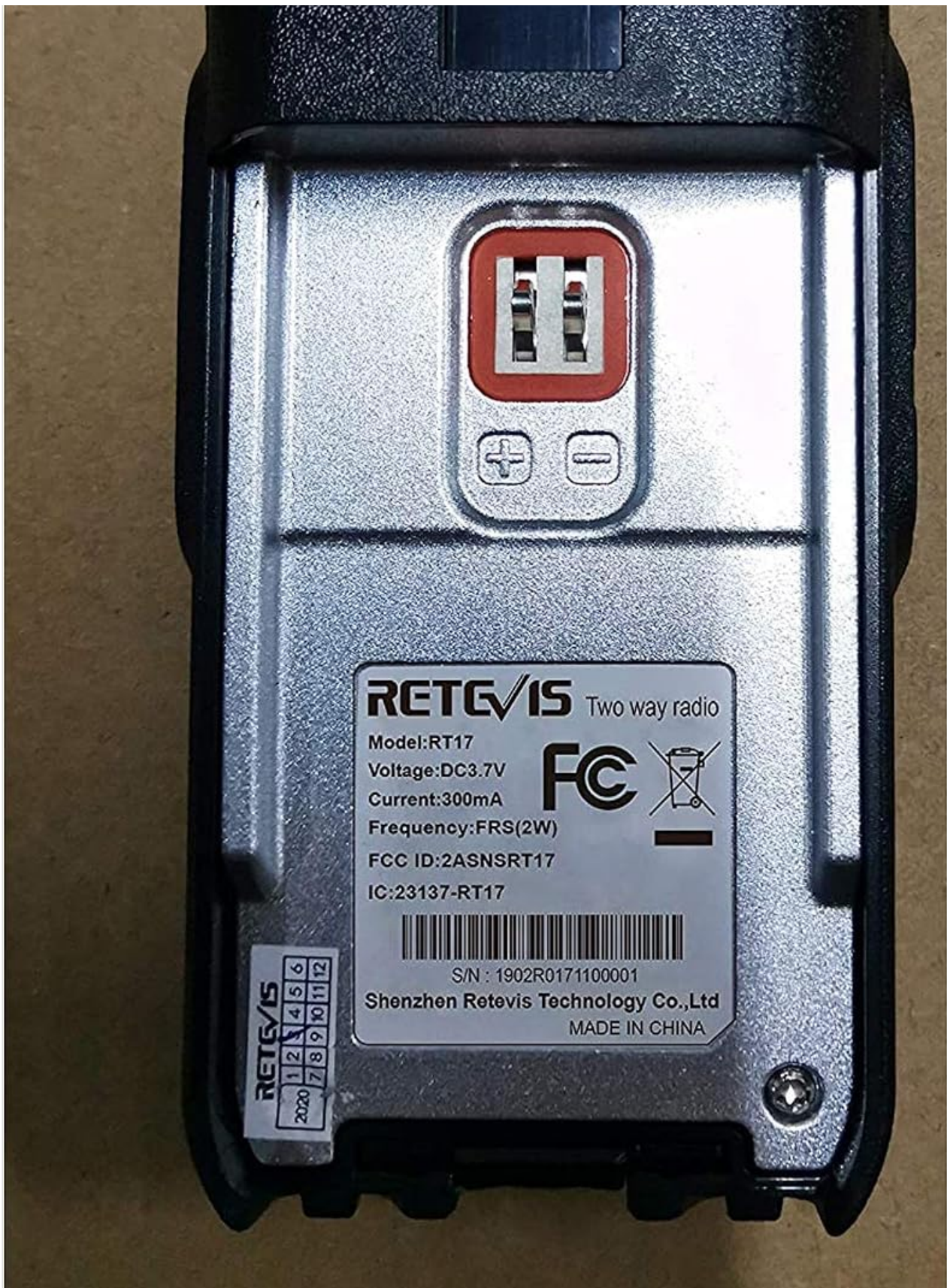
Figure 4: Rear view of the RT17 radio, displaying the model number (RT17) and FCC ID (2ASNSRT17), confirming compliance with FCC Part 95 rules.
