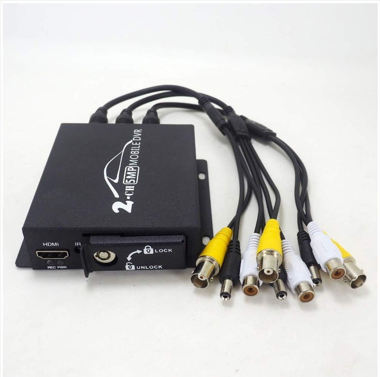
Figure 4.1: DVR with Connected Cables. This image shows the DVR unit with the power cable, two camera input cables, and an AV output cable securely connected to their respective ports.
