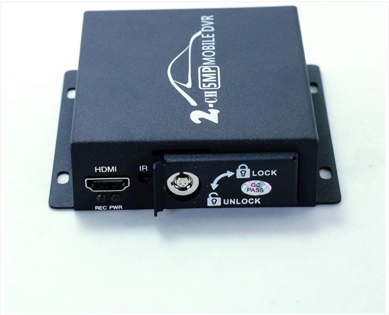
Figure 3.2: SD Card Compartment. This image shows the protective cover for the dual SD card slots, along with the key-operated lock mechanism indicating 'LOCK' and 'UNLOCK' positions.
