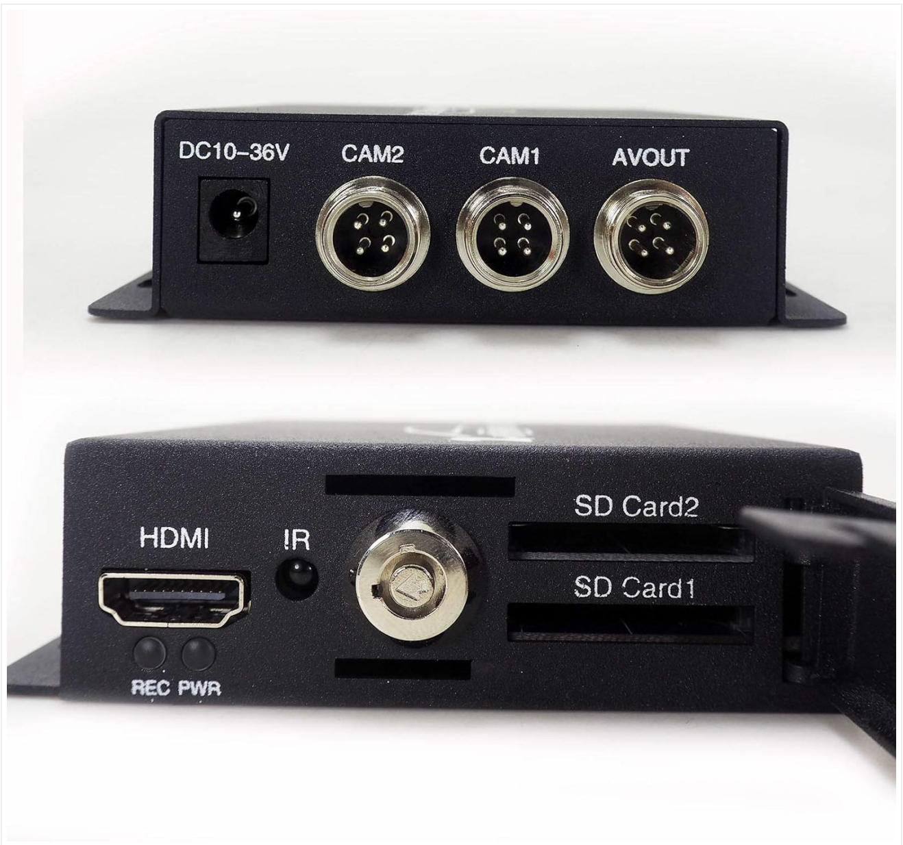
Figure 3.1: DVR Front and Side Panel Overview. This image highlights the DC power input, two camera input ports (CAM1, CAM2), AV output, HDMI output, IR receiver, REC and PWR indicator lights, and the dual SD card slots.
