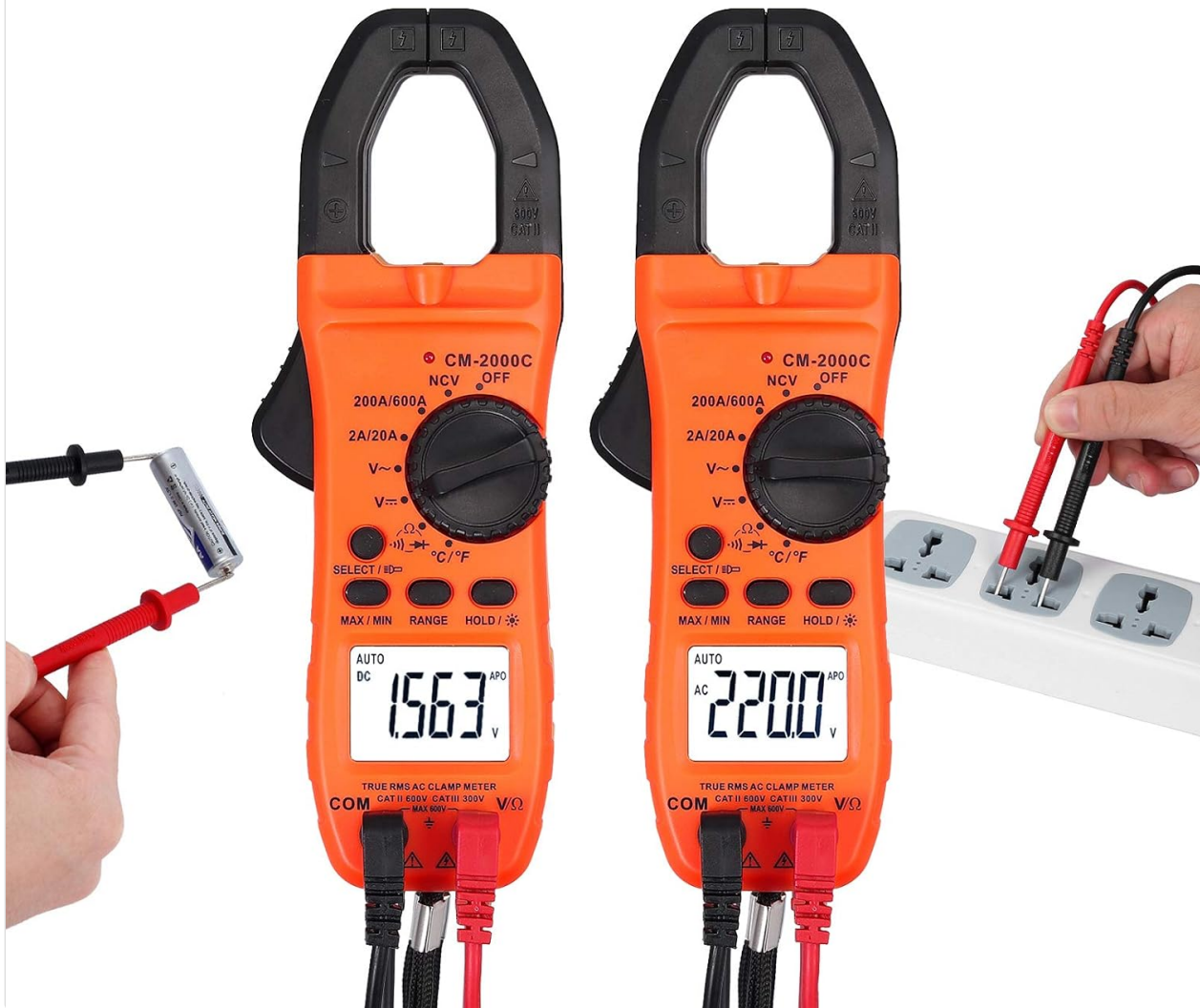
Figure 5.1: DC and AC Voltage Measurement.
