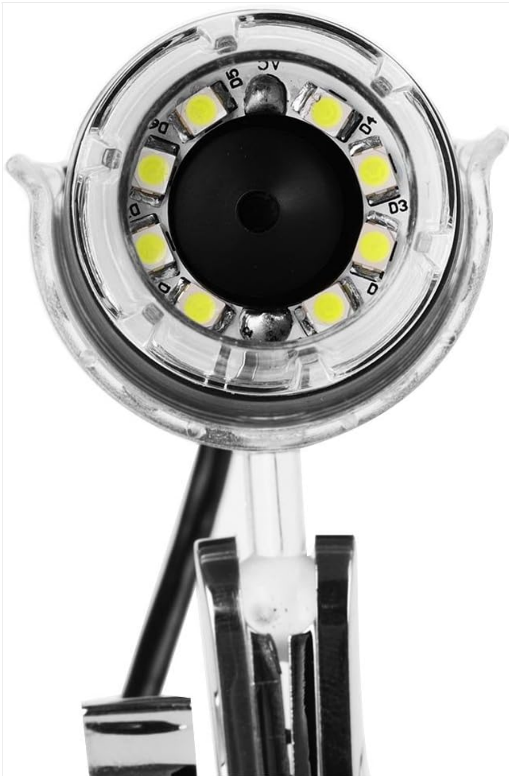
Image 6.3: The front of the microscope with its 8 LEDs illuminated, demonstrating the lighting capability for viewing specimens.
