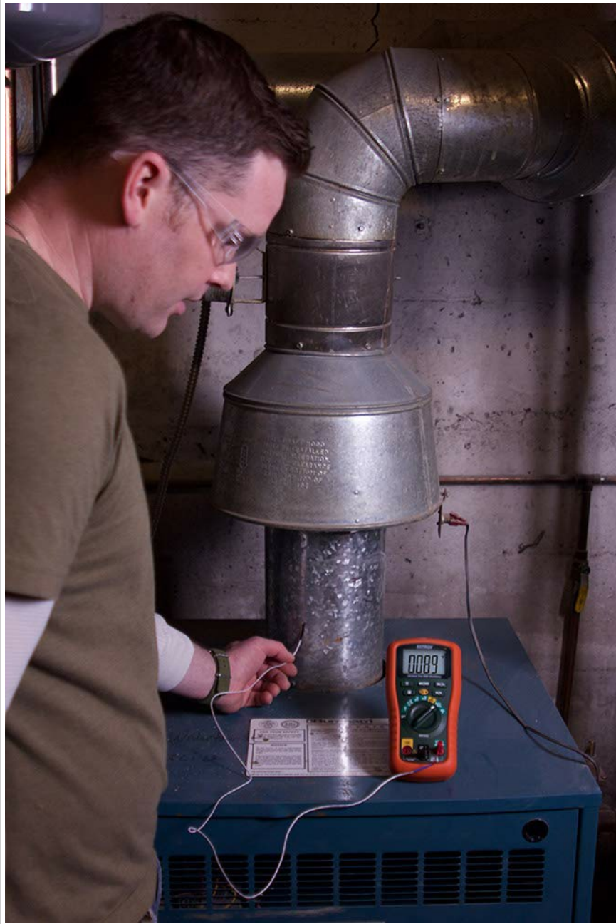
Figure 5: A technician using the Extech MM750W Multimeter with its Type K temperature probe to measure the temperature of a furnace flue, demonstrating the meter's temperature measurement capability.
