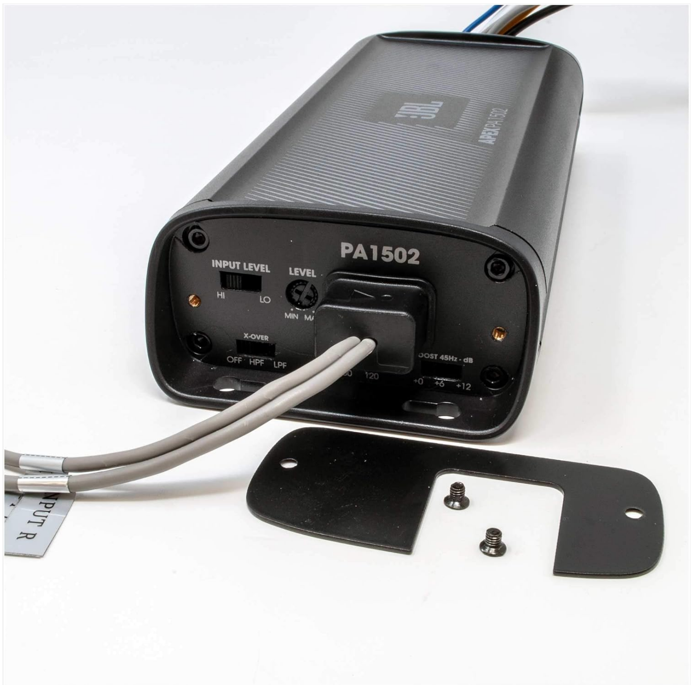
Image: Detailed view of the amplifier's control panel, illustrating the input level switch, gain adjustment, crossover frequency selector, and bass boost controls.
