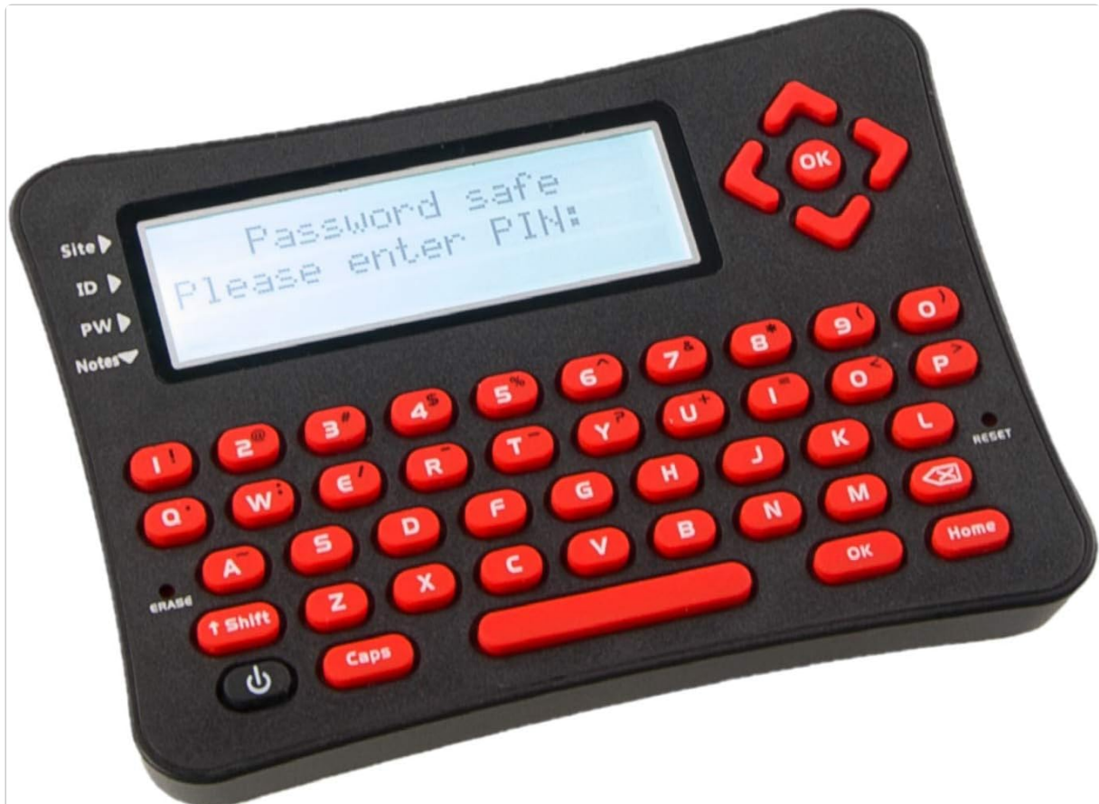
Figure 4.1: Front view of the Mindscope DigiSafe Password Vault, showing the LCD screen, alphanumeric keypad, and navigation buttons. The screen displays a prompt to enter the PIN.
