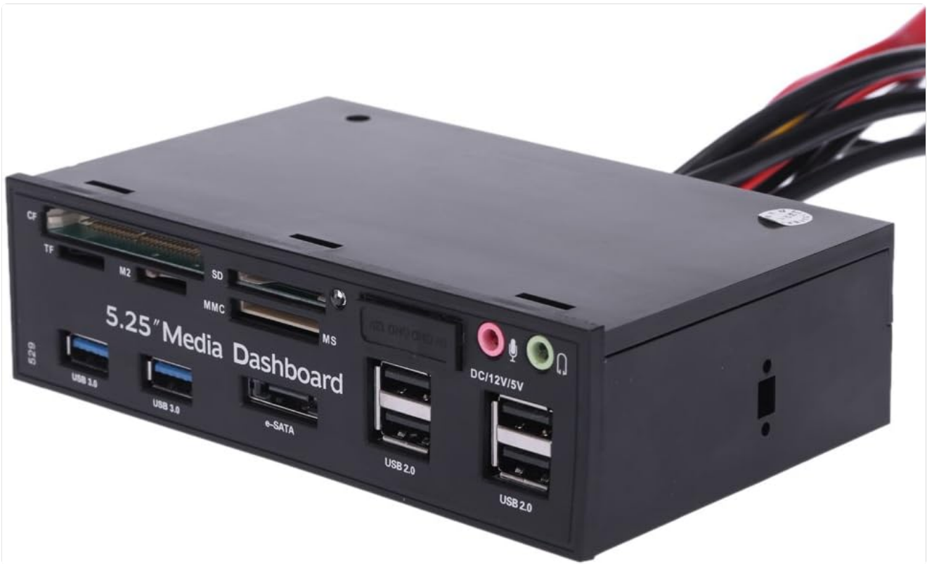
Figure 2.2: Detailed view of the front panel, highlighting the labels for each port and card slot for easy identification.
