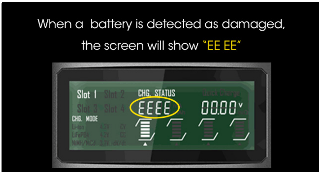
Image: The UMS4 display showing the "EE EE" error for a damaged battery.
