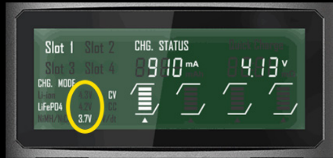
Image: The UMS4 screen showing voltage selection options (4.3V, 4.2V, 3.7V) for manual adjustment.
