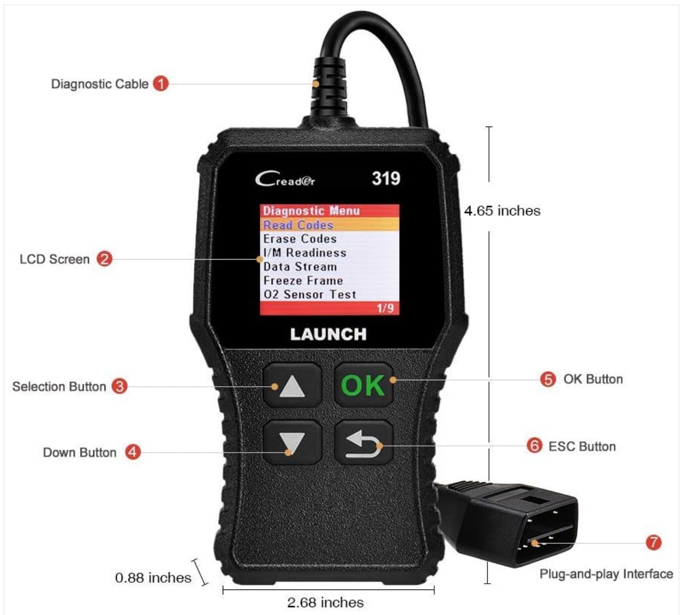
Figure 2.2.1: LAUNCH CR319 OBD2 Scanner with labeled components.
