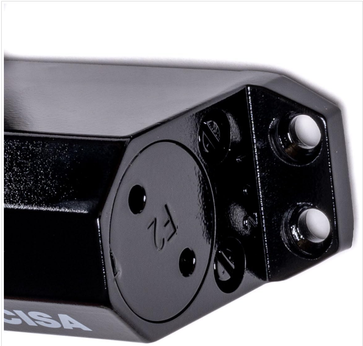
Figure 2: Close-up view of the CISA Serie 604 door closer's adjustment valves. This image shows the two adjustment valves on the side of the door closer body. These valves control the closing speed and the final latching speed.
