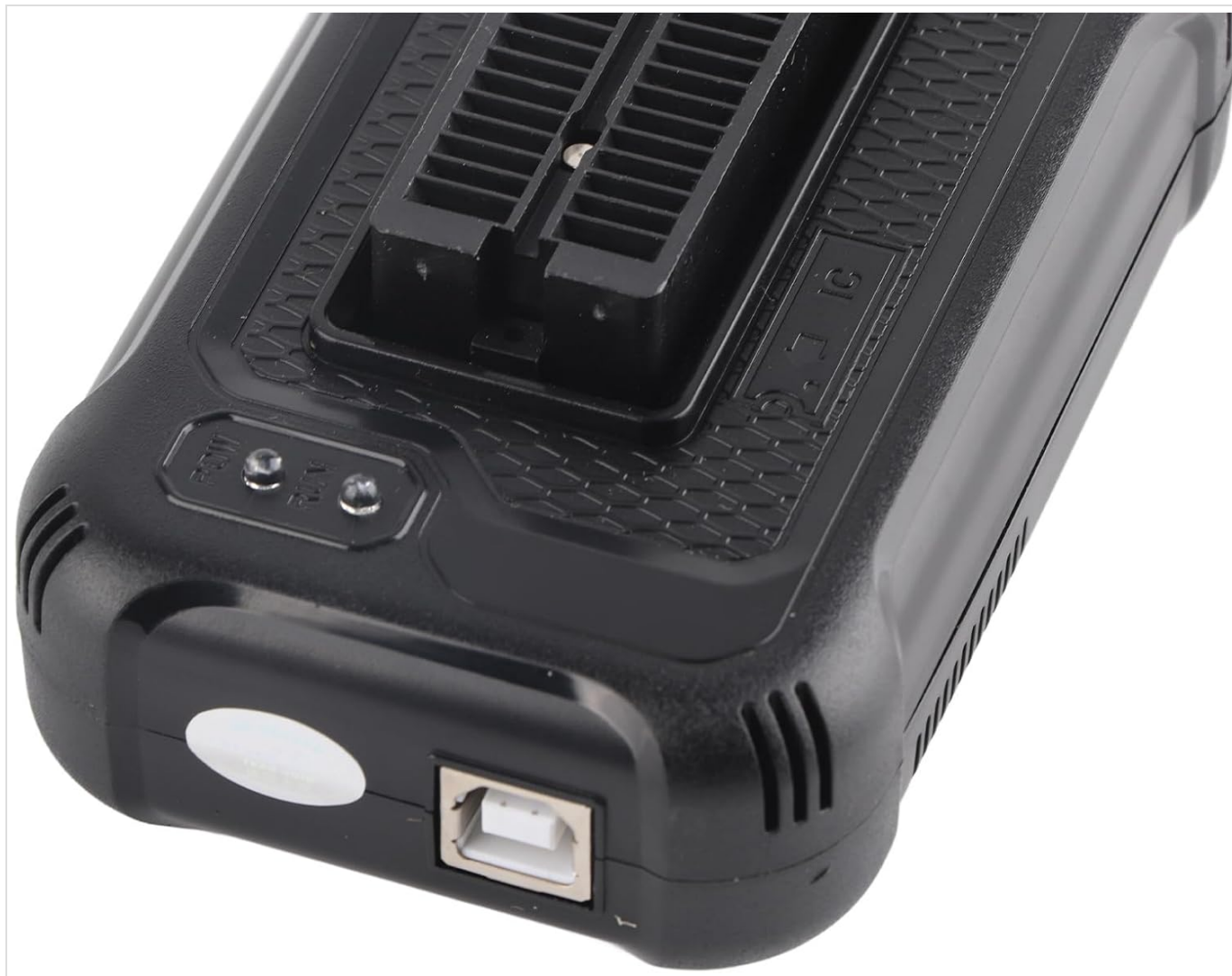
Figure 4: The USB port on the Vikye TL866II Plus programmer for computer connection.
