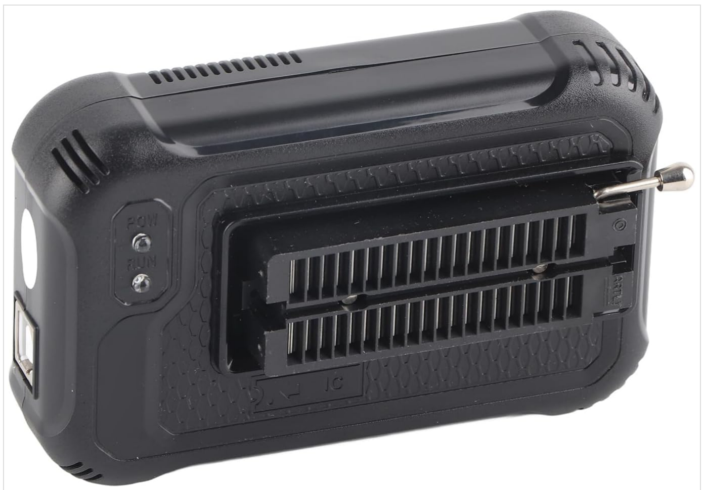
Figure 5: The ZIF socket on the programmer for chip insertion.
