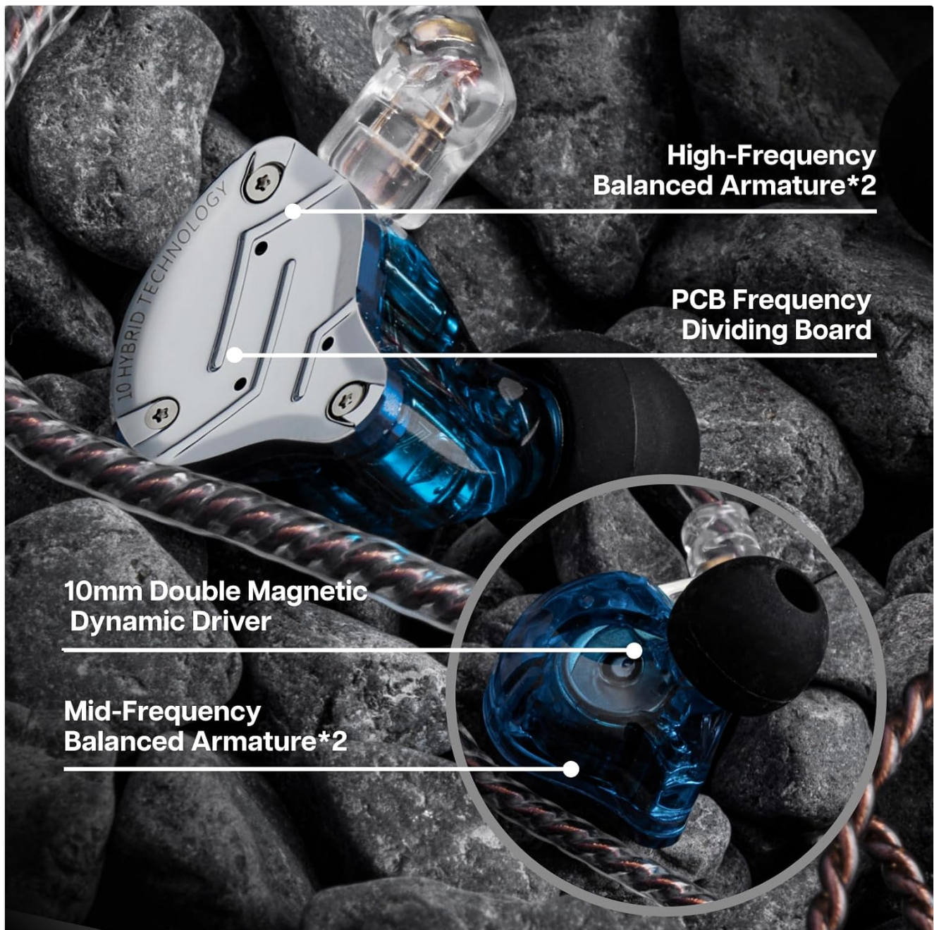
Image: Internal structure of the KZ ZS10 Pro, detailing its hybrid driver system.
